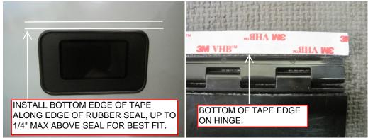
3) After verifying and marking install location remove protective paper tape strip. Carefully position the hinge in position and press firmly to seat the tape on the metal surface, lifting the flap if necessary to make sure the hinge tape is seated squarely with the metal surface. Use a towel to put firm pressure on the taped part of the hinge and slide back and forth across to fully seat and activate the tape adhesive.
